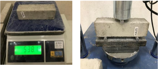
Figure 2. Measuring the unit volume weights of samples and Flexural Strength
