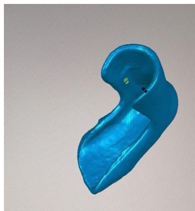
Figure 3. Processed mesh model of the reference clubfoot orthosis in Geomagic Studio after mesh repair, smoothing, and surface correction operations.
