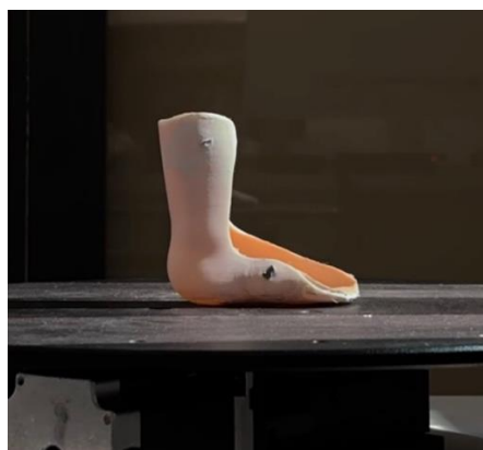
Figure 1. Positioning of the reference clubfoot orthosis on the scanning platform during the 3D scanning process.
