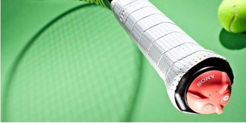
Görsel 3. Tenis raketine entegre edilen Sony Smart Tennis Sensor cihazı, (Sony Corporation, 2015)
