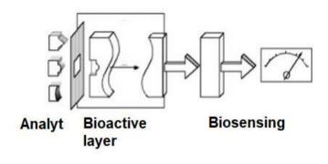
Figure 1. Principle of the biosensor.
