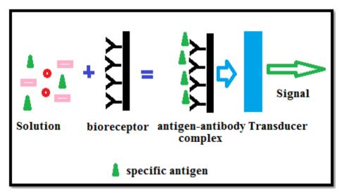
Figure 2. The working principle of the immunosensor is schematized.
