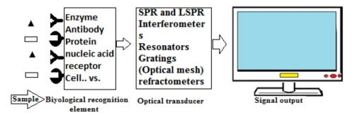
Figure 1. Schematic representation of optical sensors [19].
