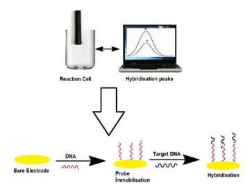
Figure 3. Working prencible of the genosensor
