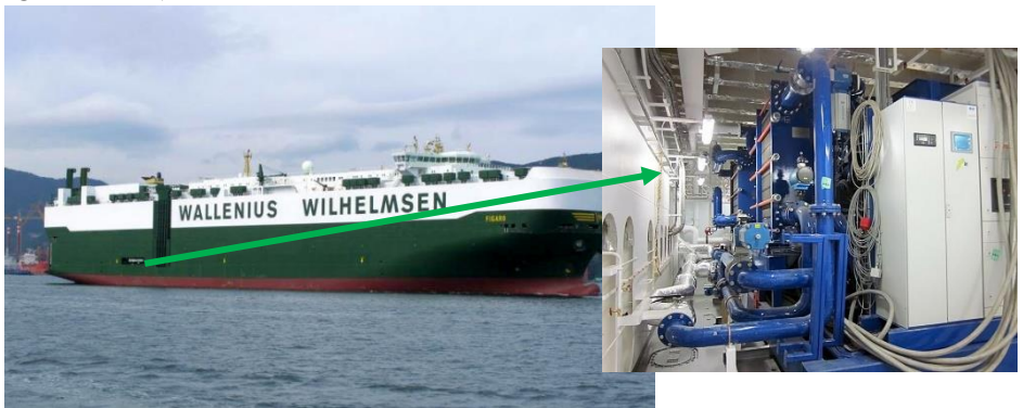
Figure 7. The MV Figaro and Opcon Powerbox ORC WHR system.
