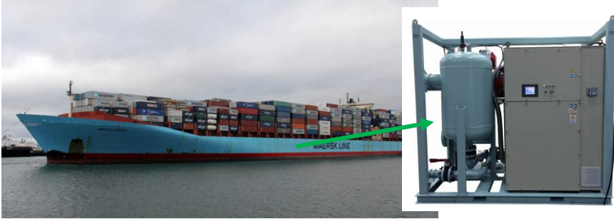
Figure 8. The Arnold Maersk and 125 kW – ORC jacket cooling water WHR.
