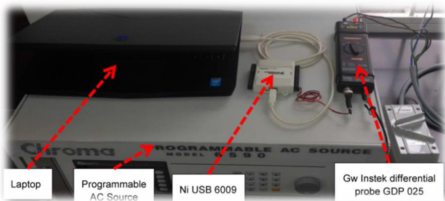
Figure 8: Experimental Setup for Fast Estimation of Harmonics [10]
