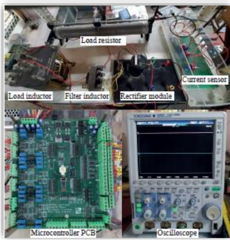
Figure 15: Experimental Setup in [17] used for Harmonic Extraction
