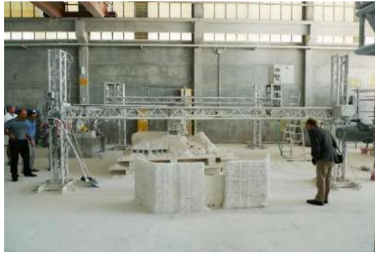
Figure 3. D-Shape 3D printing method (ESA, 2022).
