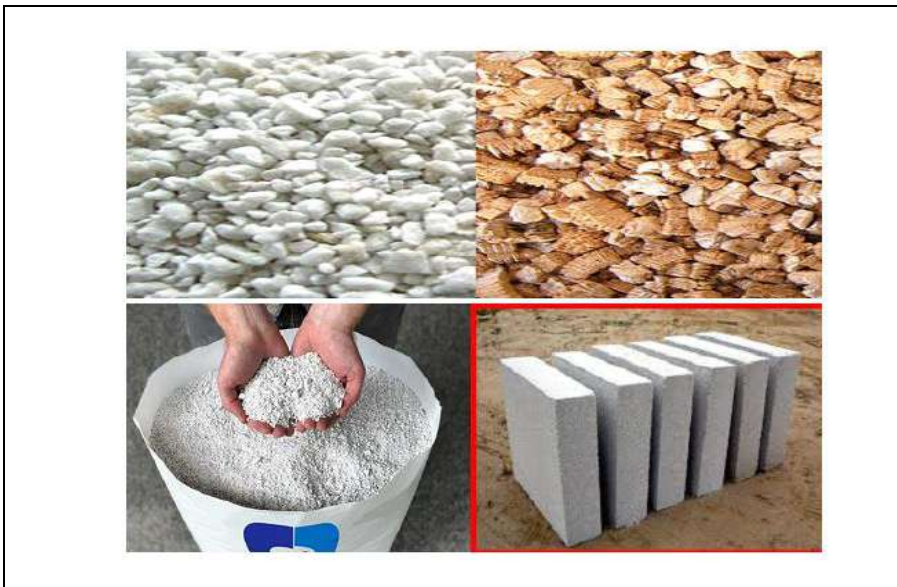
Figure 2. General grain structure formed by processing perlite mineral [1,5]
