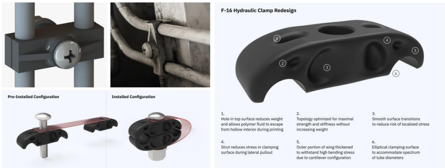
Figure 1: F-16 Aircraft Hydraulic Tube Clamps
