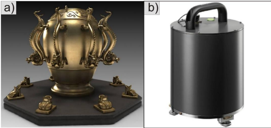
Figure 2. The oldest and newest seismometers a) The oldest known seismoscope manufactured by Chang Heng (Yan, 2007) b) The most preferred GURALP-3ESPC Feedback Broadband seismometer for new generation and seismological monitoring networks (SYY, 2023)
