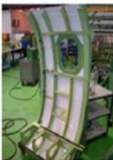
**Aircraft Door Parts and Back Panel** made of AZ31B Mg-alloy.
