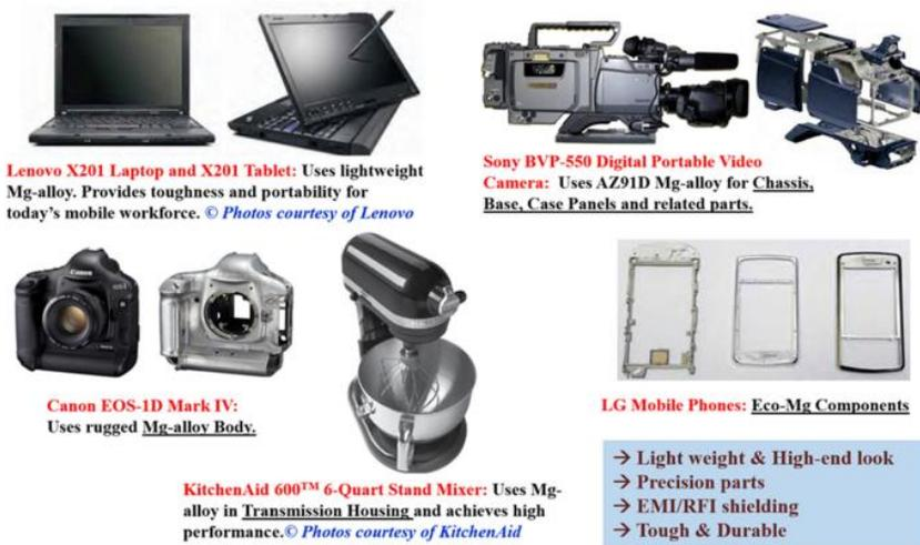
**Fig.3:** Areas of use of magnesium composites in the electronic devices
