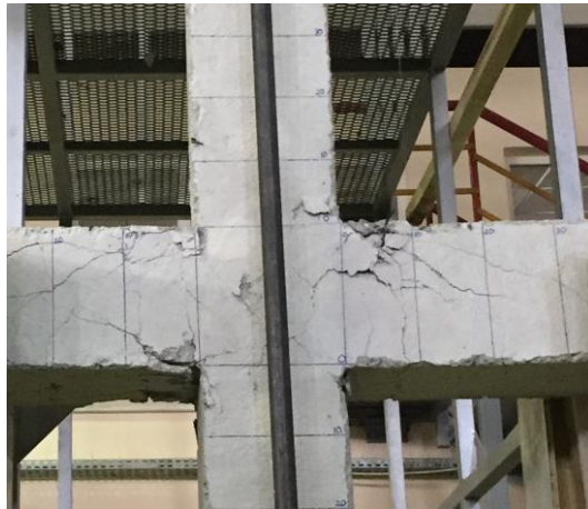
Figure 9. Flexural cracks in reinforced concrete beams [59]
