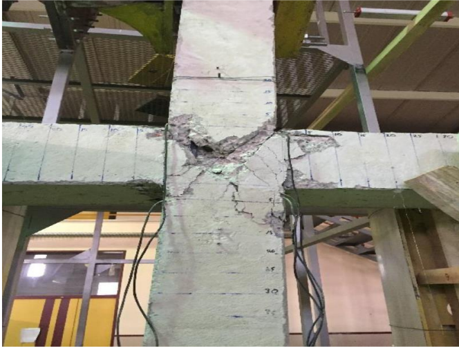
Figure 10. Cracks occurring in the beam-column joint region of reinforced concrete structures [60]
