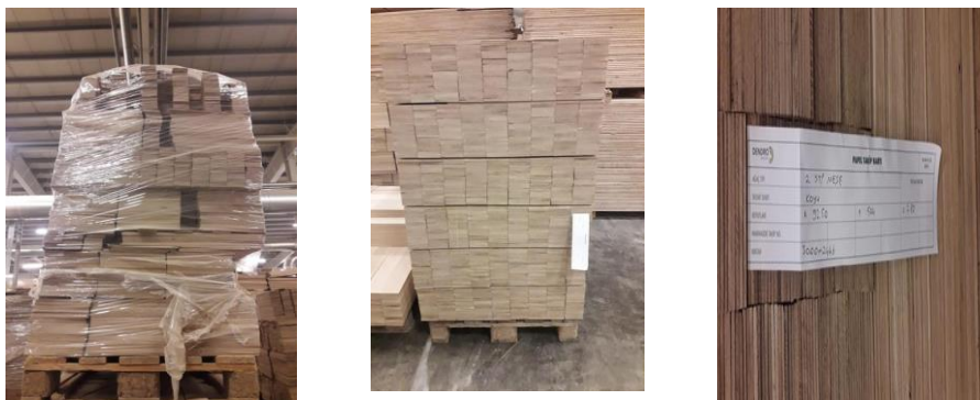
Figure 1. Comparison of veneer lamella pallet organization before and after the 5S implementation, together with the visual identification cards introduced as part of the 5S system.
