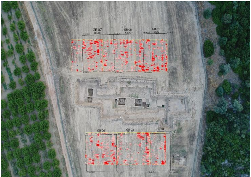
Ground-Penetrating Radar Survey Data of the Roman Buildings Unit, 2021
