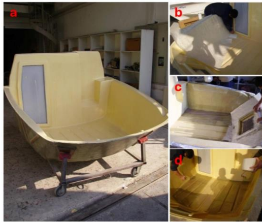
Figure 3. Boat manufacturing by hand lay-up method (Güven Tekne Ltd. Şti, Çiğli, İzmir), a) Female polyester hull mold, b, c) Fiberglass lay-up, d) Resin impregnation.
