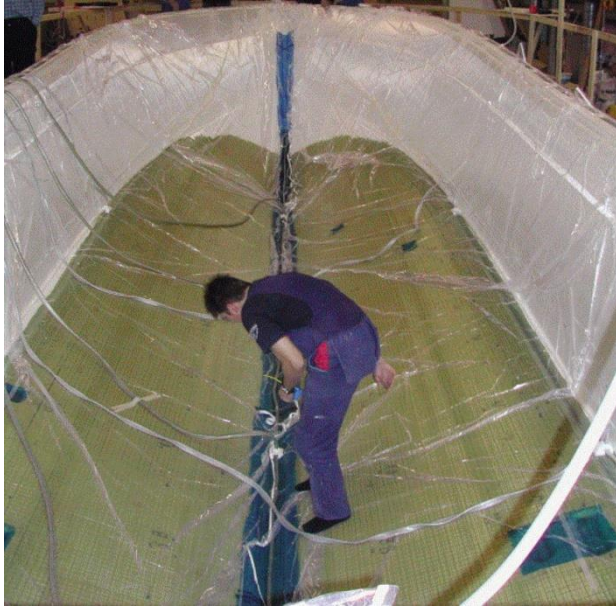
Figure 7. Production of sandwich composite boat hulls with VARIM (Technology update: Vacuum infusion,2004)
