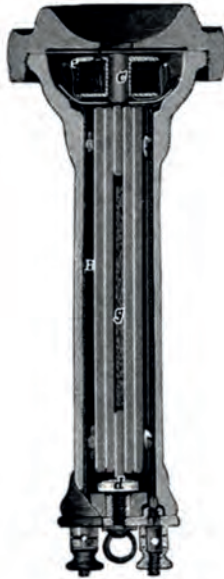
FIG. 58.—LONGITUDINAL SECTION OF BELL TELEPHONE.
