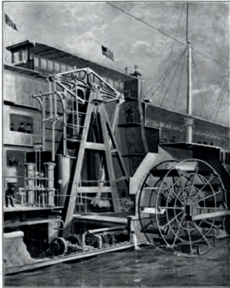
FIG. 113.—ENGINES AND PADDLE WHEEL OF STEAMER "ADIRONDACK" ON THE HUDSON RIVER.
