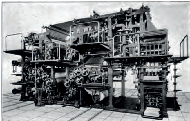
FIG. 124.—HOE OCTUPLE PRESS. PRINTS, CUTS, PASTES, FOLDS AND COUNTS NEWSPAPERS AT RATE OF 1,600 A MINUTE.
