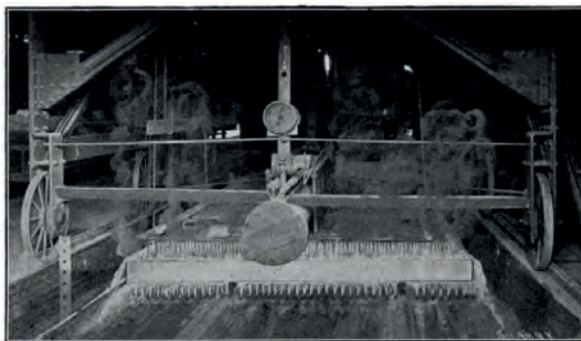
FIG. 261.—HARDENING THE PLATE BY JETS OF WATER.
