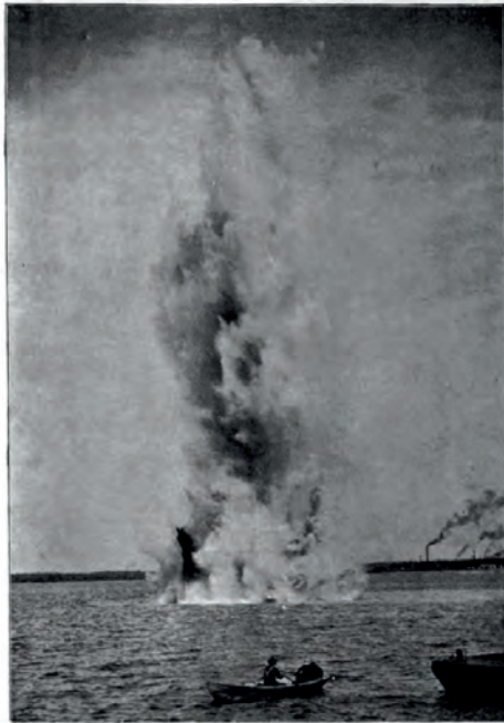
FIG. 284.—EXPLOSION OF A MINE. BASE OF WATER COLUMN, 100 FEET WIDE, HEIGHT, 246 FEET.
