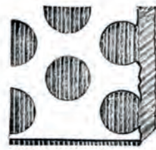
FIG. 65.—ENLARGED DETAIL OF PLANTÉ PLATE.
