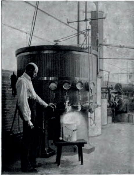
FIG. 301.—COMMERCIAL PRODUCTION OF LIQUID AIR.
