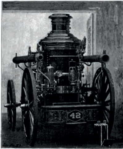
FIG. 91.—STEAM FIRE ENGINE WITH WATER HEATING ATTACHMENT.
