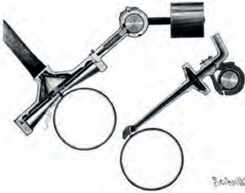
FIG. 191.—THE GRAPHOPHONE, RECORDING AND REPRODUCING DEVICES.
