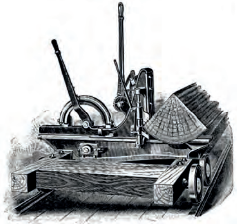
FIG. 243.—METHOD OF SHAPING AND HOLDING LOG FOR QUARTER SAWING.
