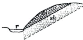
FIG. 11. Diagram Illustrating Conditions favorable to a Landslide
