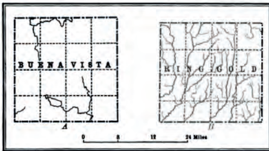
FIG. 50. Drainage Maps A, an area in its infancy, Buena Vista County, Iowa; B, an area in its maturity, Ringgold County, Iowa
