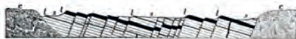
FIG. 315. Section of Triassic Sandstones of the Connecticut Valley ss, sandstones; ll, lava sheets; cc, crystalline igneous and metamorphic rocks
