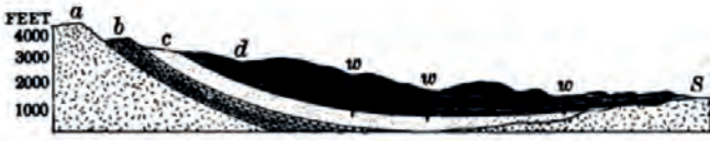
FIG. 29. Section across South Dakota from the Black Hills to Sioux Falls (S), Illustrating the Conditions of Artesian Wells
