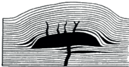
FIG. 247. Section of a Laccolith
