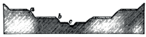
FIG. 75. River Terraces of Rock covered with Alluvium c , recent flood plain of the river. To what processes is it due? Account for the alluvium at a and b and on the opposite side of the valley at the same levels. Which is the older? Account for the flat rock floors on which these deposits of alluvium rest.
