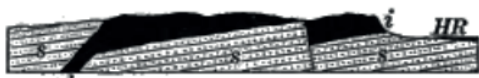
FIG. 243. Diagram of the Palisades of the Hudson i , intrusive sheet; s , sandstone; d , feeding dike; HR , Hudson River
