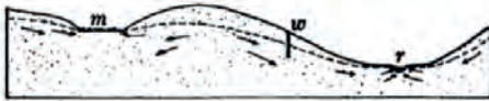
FIG. 24. Diagram Illustrating the Relation of the Ground-Water Surface to the Surface of the Ground
