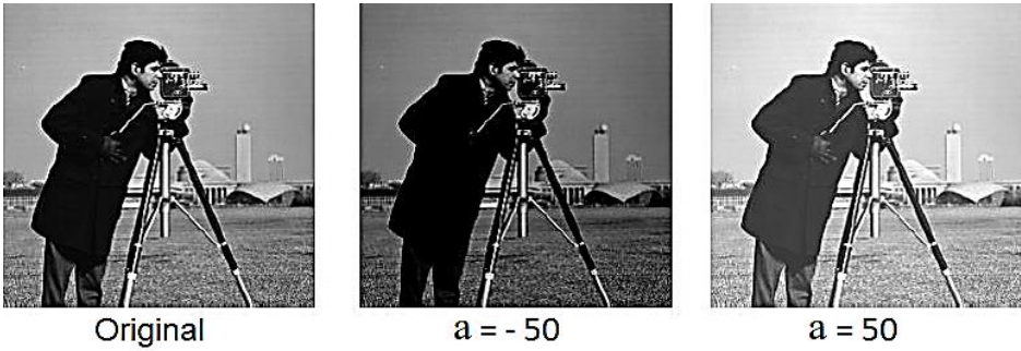
Figure 7. Light and dark states with the original image whose brightness has been changed (Gonzalez, 2009)
