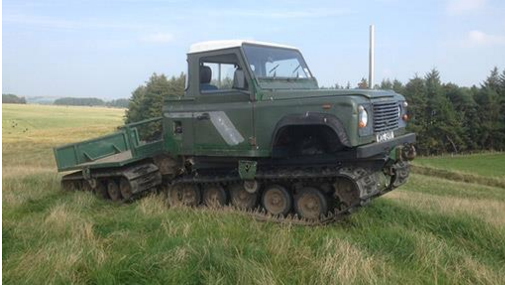
Figure 6.29. An off-road vehicle from a combination of old Volvo personnel carrier and Defender 90 65
