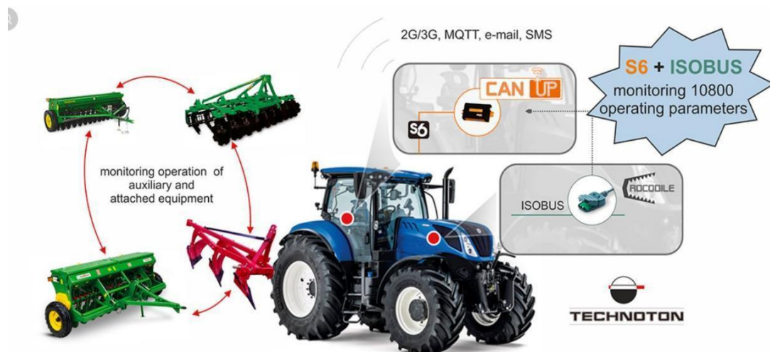
Figure 2.13. ISOBUS protocol implemented in agricultural machinery telematics
