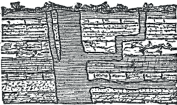
Fig. 12.—Dike with regular branches.
