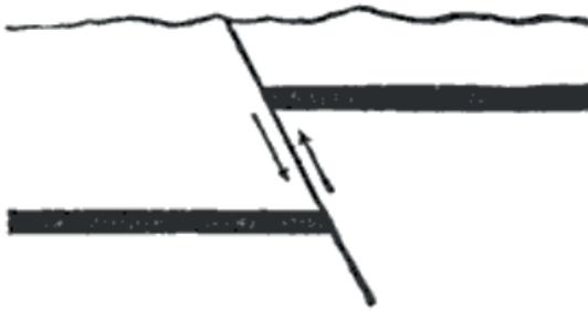
Fig. 29.—Section of a reversed fault.
