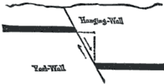
Fig. 28.—Section of a normal fault.
