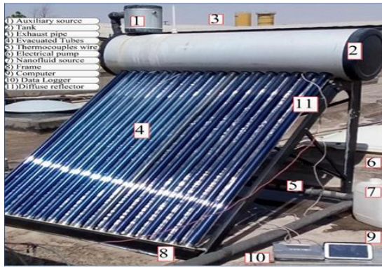
Fig. 3. The experimental set up of evacuated tubes solar collector (Ghaderian and Sidik 2017).
